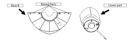
2. When assembling the body of the heater, insert the four raised parts of Base B into the corresponding holes of Base A. There are two joints on Base B. Base B must be inserted into Base A until a "click" is heard.
